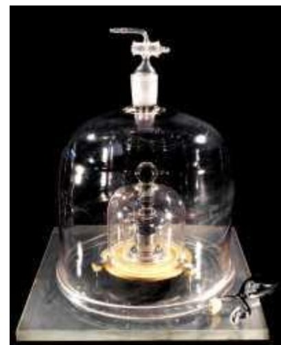
The International Prototype Kilogram. There are also six official copies stored in the same vault and additional copies around the world.
